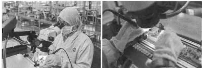
Manual soldering using a microscope
